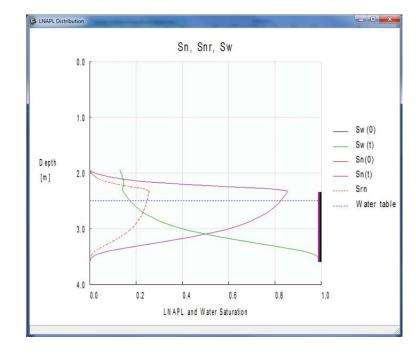
Modeled LNAPL saturation curves at peak measured LNAPL thickness (Sn (0)) in the MW-59 area (1.25 meters, or 4.1 feet shown as vertical bars at the right of plots) are:
